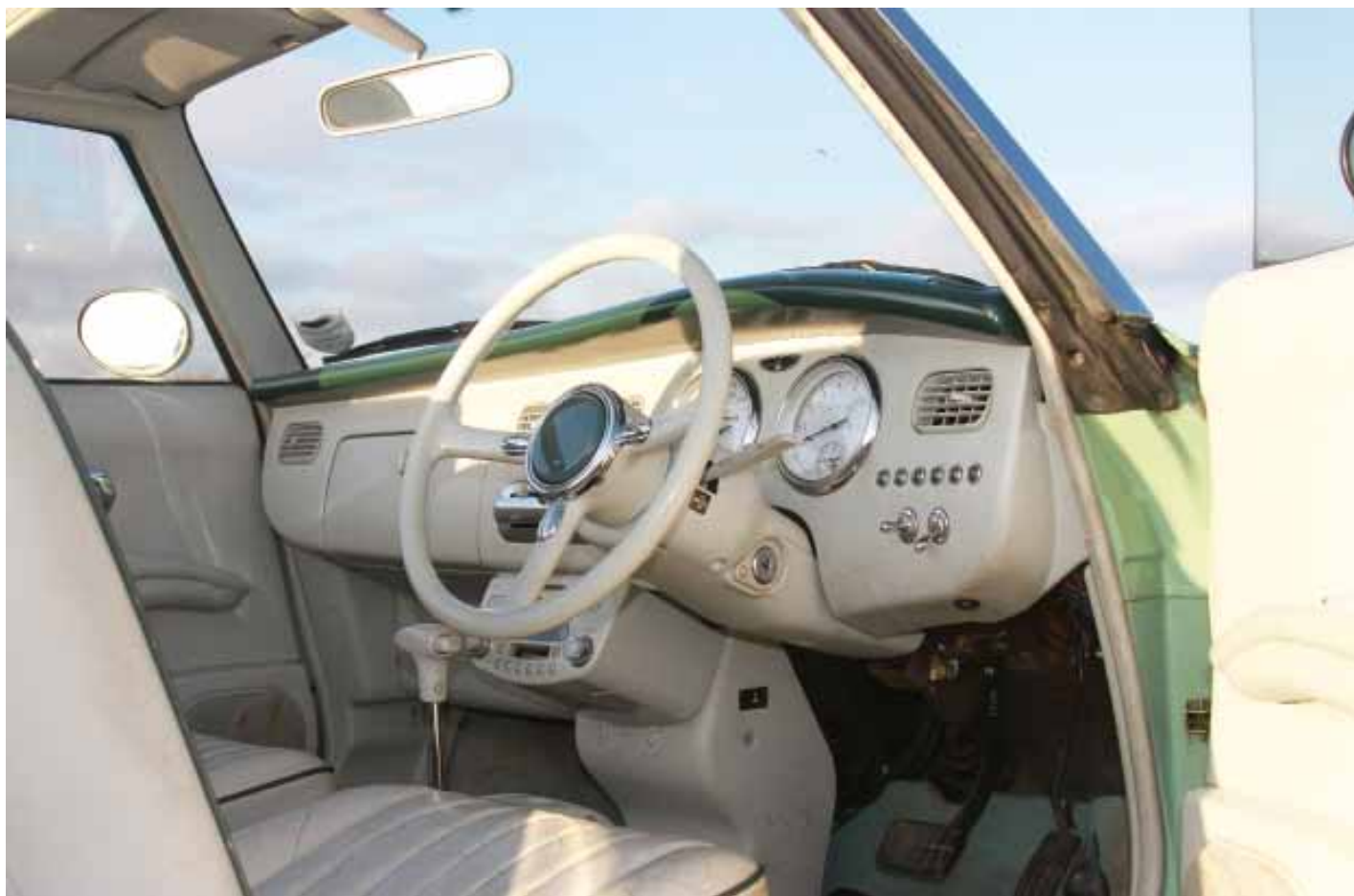
The Figaro's interior is as beautifully styled as the exterior. Initial issues are a cracked top to the dash, indicators that are temperamental, a non-functioning electric window and a handbrake lever that's been wrapped up in insulating tape.
