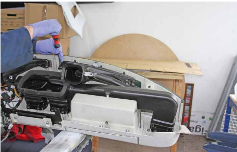
22 Enjoying the comfort of now working on the bench, our next task was to remove all of the plastic pipework for the heater and fresh air circulation system.
