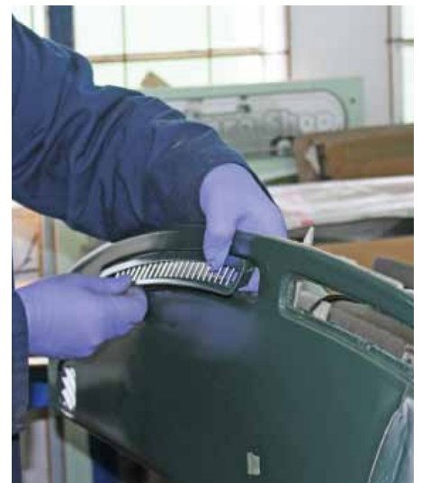
23 Before undoing the many screws holding the green dash top to the dash itself, we had to carefully pop out these grilles, which are easily damaged.
