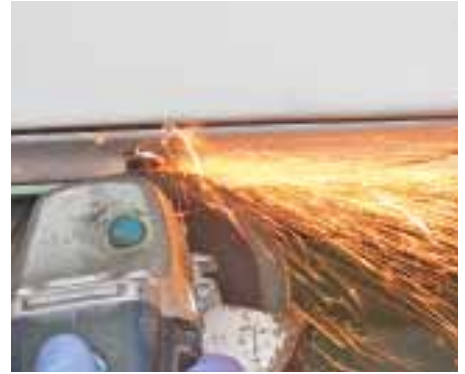
3 So now we had to remove the door card to examine other components in the system. There are four screws in cup washers holding the bottom edge of the door card to the frame. One was so rusted that Ant had to cut a slot in the head and use a flatblade screwdriver to turn it out.
