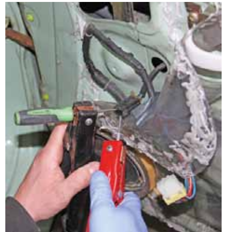
5 Now we could test the window motor, but running power directly to it had the window opening and closing on demand. So the only suspect left was the relay box.
