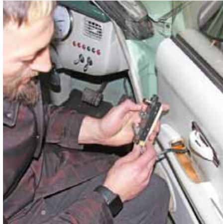
2 ...and tried another switch from their parts shop. That gave the same problem though, namely that we could hear the relay click, but the window did not move.
