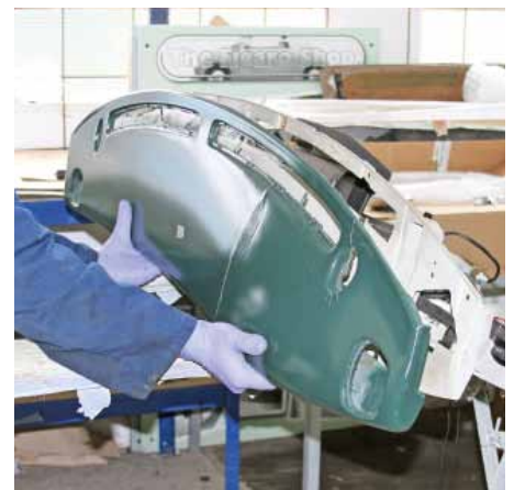
25 Finally the dash top itself could come off. We were surprised to discover that it was actually metal underneath and the crack was only in the top shell.
