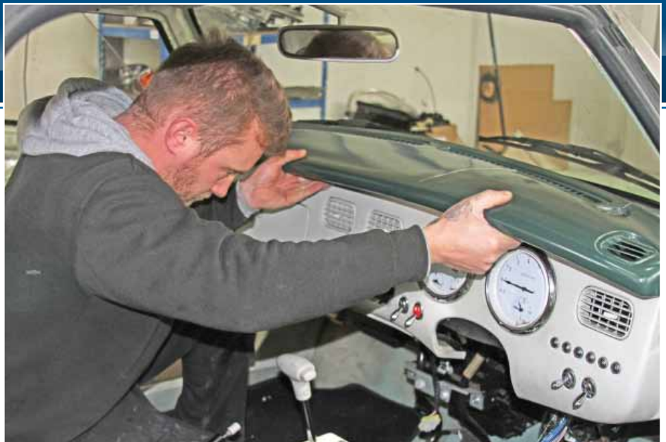
21 Finally the dash could be manoeuvred out of the car and laid on a padded bench. Note that the rev counter has for some strange reason stuck at 1000rpm!
