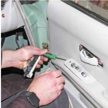
1 One of the jobs on our list was that the electrically-operated window in the driver's door would no longer operate. So Toby flicked out the switch unit...
