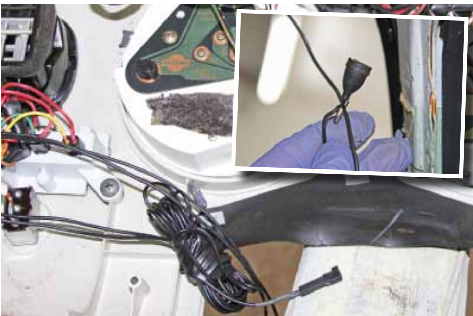
24 Aftermarket alarms are often more trouble than they are worth, so we also took out miles of alarm wiring and the microphones. The alarm's 'brain' had already been taken out on our car, so it was not working anyway.
