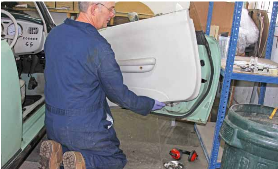
4 The card could then be levered out of the retaining clips and twisted up and out after removing door pull and handle screws and disconnecting the window switches.
