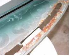
2 This is the underside of the old dash top, showing the metal clips that are folded over the dash structure to hold it in place. The metal top will support the fragile plastic section pictured in step 1.
