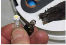
20 One final job to be done at this stage before we could begin putting the Figaro back together was to replace the bulbs in the dash instruments with brighter LEDs. As well as the six instrument bulbs...
