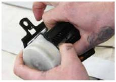
**18** Turning the spindle against the spring pressure without the belt inserted meant that the retracting pressure could be increased, but we didn't want to make it so tight it was uncomfortable.
