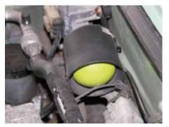
222We had already removed the wiring and microphones to the nonfunctional aftermarket alarm, and now we could remove the alarm's siren from under the bonnet too.
