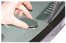
Reassembly then really was a reversal of the dismantling process, though the cover at either end over the securing nuts and studs had to be stuck down with silicone because of the thicker leather.
