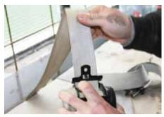
**14**With the seatbelt and its mechanism on the bench, the first job was to pull the belt out as far as it would go. A bit of fabric cleaning wouldn't go amiss, but that can be done later on the car.
