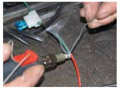
23 Unfortunately the rear fog light that had been fitted when the car was imported to comply with UK regulations had taken its feed from the alarm wiring, so Ant had to solder in a new feed.
