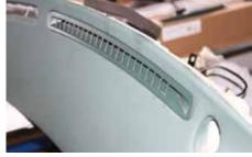
4...would have made the gap too narrow for the plastic demister vents to clip into place. These are quite vulnerable where the thin cross-piece vanes are located, so you don't want to force them.
