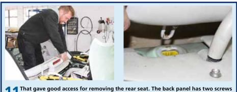
That gave good access for removing the rear seat. The back panel has two screws at the bottom, then pulls out and up, but these locating pegs were very tight.
