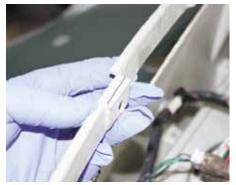
**1** The plastic dash structure itself is quite brittle, presumably not reacting well to the aging process. Ours was cracked in a couple of places, but this break was not in a critical position.
