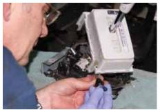
21 ...there was also one for the gear selector and another for the aircon. LEDs only function in one direction, so we reattached the battery and checked they worked before final reassembly.
