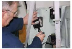
**1**3 All of this was to gain access to the mechanism itself. Before removing it, we did make a precautionary check that the locking mechanism was working correctly by tugging sharply on the belt.
