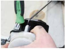
**16** With the spring pressure removed from the equation in this way, the end of the seatbelt could then be prised gently from the spindle with a second pick.
