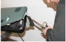
**7** This area is quite a tight fit against the screen pillar, so once the adhesive had fully cured, Ant sanded off any excess that had been squeezed out.
