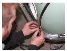
24 And finally, we were missing the back of this brightwork. Fortunately The Figaro Shop had a new replacement on the shelves and it clipped into position.
