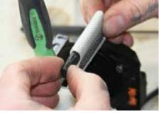
**17** Taking great care not to damage the material with the pick, the plastic end through the belt's loop could be removed and then the belt pulled through the other way and out of the spindle.
