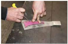
5 We saw last issue how the plastic dash was crumbling slightly at the ends where it was secured to the car. This is so common that The Figaro Shop have a template for repair sections in this area.
