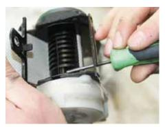
**15** With the seatbelt unwound to its full bextent, the mechanism was under tension and trying to pull it back in, so Ant pegged it with a pick through this hole.
