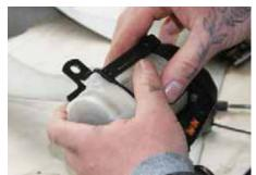
**19**Ant decided that one full rotation of the spindle was all that was needed, then he threaded the belt back though, inserted the plastic plug and wound it all carefully back in.
