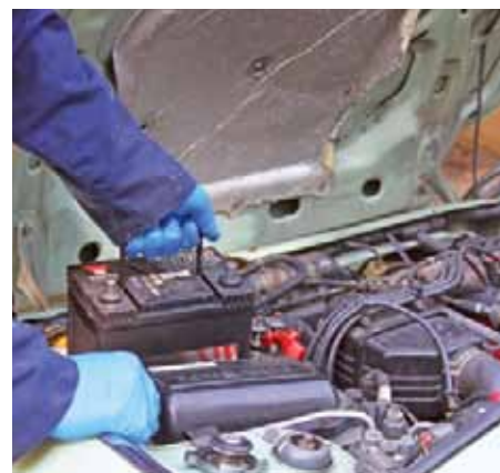
5 The engine bay is so cramped that items had to be removed one at a time to gain access to the hoses and the radiator. Removing the battery was a safety measure as well as to provide elbow room.
