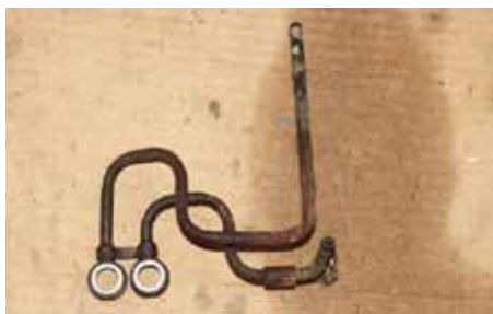
9 The other end of those rubber oil-coolant pipes attach to this steel pipe assembly which in turn is secured to the gearbox with banjo bolts. The metal pipes were rusted, but not terminally so.
