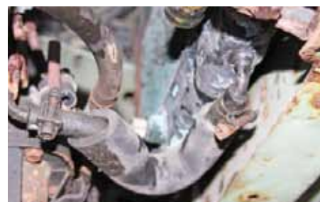
8 There is an oil cooler in the bottom of the radiator for the gearbox oil, pictured here from underneath the car. The rubber pipes to this are simply a push fit held on with regular hose clamps.
