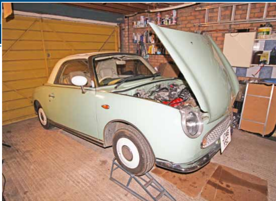
4 Back home, the Figaro was lifted rather than driven onto ramps, which explains how one was placed the 'wrong' way round to ensure the car could not roll off by accident.
