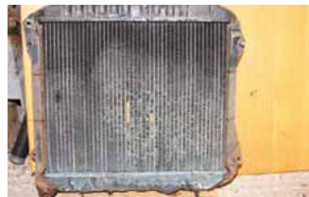
11 The old radiator came out with just one sheared bolt. It really was in a very sorry state, with large sections where the cooling fins had disappeared and others falling off at the slightest touch.
