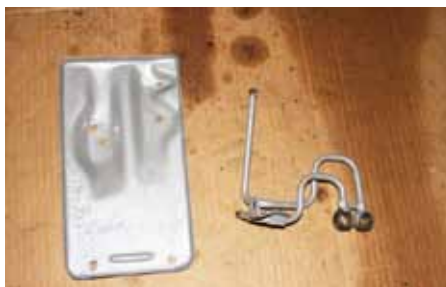
10 Simon had the battery tray and the pipes blasted and powder coated, after first wrapping the unions in tape to protect them. The blasters used a low pressure on the potentially delicate pipes.
