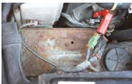
6 This showed that the battery tray had plenty of surface rust. The tray itself was painted grey rather than body coloured, and was secured to the chassis rail with bolts. The rail beneath was sound.
