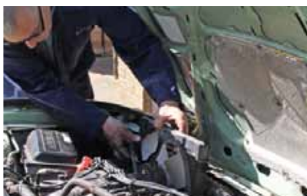
7 Simon took the fan assembly off the radiator while it was in the car. That gave greater access and visibility to study the task in hand, but made the removal more difficult than it needed to be.
