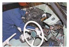
**15** Finally the whole heater unit could be lifted carefully out of the car, taking care not to let any residual water still trapped inside pour out and onto the carpet. Oh for the easy access of an engine-bay heater on a Midget or MGB!
