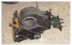
**16** And this is the reason for it all. Note the two plastic pipes to the left that poke through the bulkhead and take hot coolant to the heater and then return it to the engine bay. Or rather, note the one stub and the broken remains of the other!
