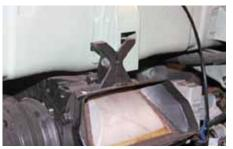
**1** With the dash removed, it was then a matter of searching around the heater unit to locate and identify all the fixings. There was this plastic hook at the top that grips a bracket on the bulkhead and is secured with a single bolt.
