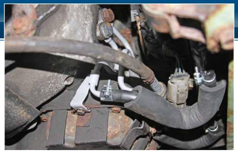
**5** And here are the powder-coated pipes fitted to the transmission, taking the oil to **b** rubber pipes that connect with the oil cooler in the bottom of the new radiator. Note the new pipe clips on the rubber hoses instead of the old wire ones.
