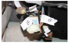
**7** With so many electrical connections to break, Simon adopted a fool-proof method, labelling each side of every connection with masking tape and a unique letter. A goes with A, B goes with B and so on – simples!
