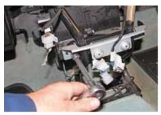
**14** So the bracket had to come off too. It heater unit out, though with more flexing of the plastic than was comfortable. At least it meant the rigid lines to the air-con unit did not have to be disturbed.
