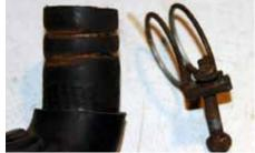
**3**Nissan used twin-wire clamps on all hoses, but these do tend to cut into the rubber when tightened. Simon was happy to reuse them on low-pressure air feed hoses, but used genuine Jubilee clips on the new coolant pipes instead.
