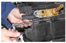
**17** With the heater unit on the bench, work could start on separating the two halves of the plastic casing. Each bolt was checked as it came out – if any had been a different length to the others, its position would have been noted.
