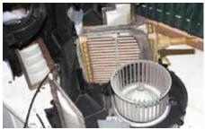
**18** There was one fixing bolt hidden deep in a recess by the fan, but after that had been found it just needed the rod for the defunct valve to be removed and the unit could be opened to reveal the heater matrix that needed replacing.
