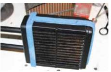
21 So Simon used new self-adhesive foam strips to wrap the new heater matrix, and also to replace the crumbling foam on the various directional flaps as well as the fan. This was slightly thicker than ideal, but did the job OK.
