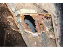
4 Pulling off the fibreglass revealed this hole in the metal. The sill structure was described in the introduction – that large hole is in the horizontal section of the central panel where it leads inwards to the inner sill/floorpan before folding down to a flange and being spot welded to them.
