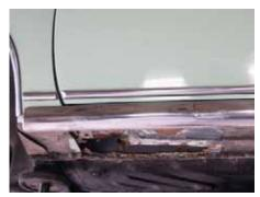
5 And this was the full extent or the missing metal after Alan had cut And this was the full extent of the ruthlessly back to sound metal - this saw a large chunk of the outer sill cut away too.
