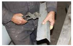
Finally moving on to the reconstruction stage, Alan first made the repair section for the central panel, punching holes on the flange for plug welding to the floor.
