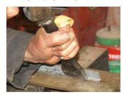
Next task was to make up a repair section for the outer sill. Here Alan is using a blunted chisel to form the step at the bottom that will wrap around the 90° bend at the bottom of the central panel.
