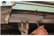
9 With the flange clamped in place, the rest of the repair section could be tweaked until it was resting snugly against the remains of the original.
