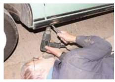
The first job was to clean off the 2 underseal that had been applied to disguise the 'repair.' We would later have to remove the stainless trim along the side of the sill too, but we didn't know that yet. Fortunately it popped off the plastic retaining lugs without issue.
