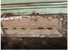
13 And here it is, welded into position and requiring final finishing before being protected against rust. Note the plug welds along the bottom of the rib joining the two repair sections together.
