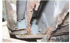
Fortunately, the corrosion was all at the bottom of the panels, and the rest of the structure was in perfect condition, giving Alan something to weld to. Here you can see the inner sill on the right and the outer sill curving under on the left.
