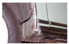
Further forward, the bottom of the inner wheelarch was unaffected. Here the wheelarch liner is folded out of the way to allow inspection. The front wings are plastic, so the bottom of that could also be eased out of the way.
