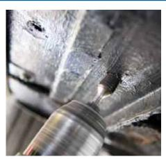
Having seen inside the panels, we had a good idea of where to drill the holes; two were required, one either side of the central membrane of the three part sill.
