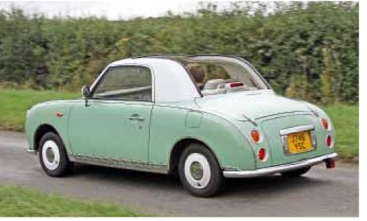
Luggage space is accessed via the lifting panel that houses the rear number plate. The bigger panel on top flips up when you raise or lower the roof to provide stowage for that.
