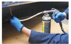
With the spray gun hooked up to a container of cavity wax and the compressor cranked up, the flexible tube was inserted in both directions and pulled slowly back out while pulling the trigger.
