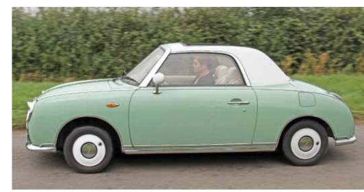
The roof sides remain in place when the soft top is stowed. This limits buffeting while still offering open top motoring, but the thick panels do restrict rear three-quarter vision.
