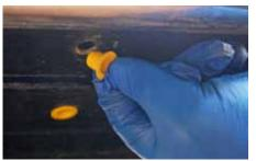
Finally, those yellow plugs closed off the holes. An extra dab of wax around the hole edges before they went in should help to stop rust from forming around the cut panel edges too.
