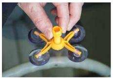
The resin is applied through this tube, then a plunger screwed down to force it in. The change was not massive and we suspect it had been done already, but at least we knew it would not get any worse.
