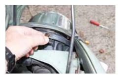
12 Finally the C-clips went back on to hold the eyelid and lamp to the body. Our thanks to the Figaro Shop for their online video explaining how these eyelids should be secured.
