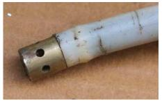
This is the spray nozzle we would be using, connected to a flexible pipe. With a number of holes in the nozzle's sides, the wax will spray out in a fan pattern to ensure 100% coverage.
