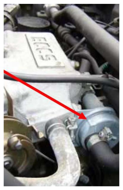
The valve is located at the back of the engine on the ECCS as below.
