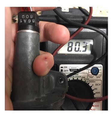
Below shows it when cold and the valve is slightly open. If its not cold you could put the valve in the freezer for about five to ten minutes which should open it.
