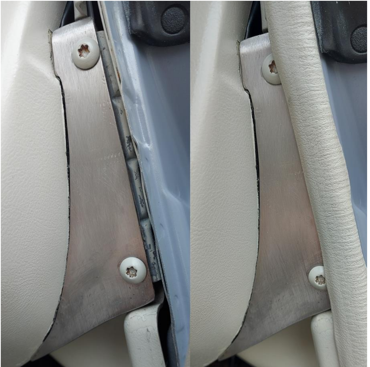
Shaped Stainless bracket attached.
